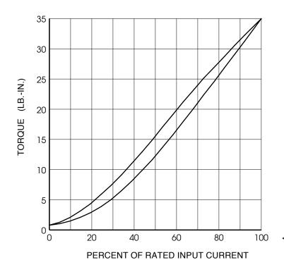
CHARACTERISTICS - With no electrical excitation, the input shaft & output shaft freely rotate. With electrical excitation, the input shaft becomes coupled to the output shaft. Torque is proportional to input current (see torque graph), and independent of slip RPM. While the load torque is less than the output torque, the clutch drives without slip. When the load torque is increased, the clutch will slip smoothly at the torque level set by the coil input
