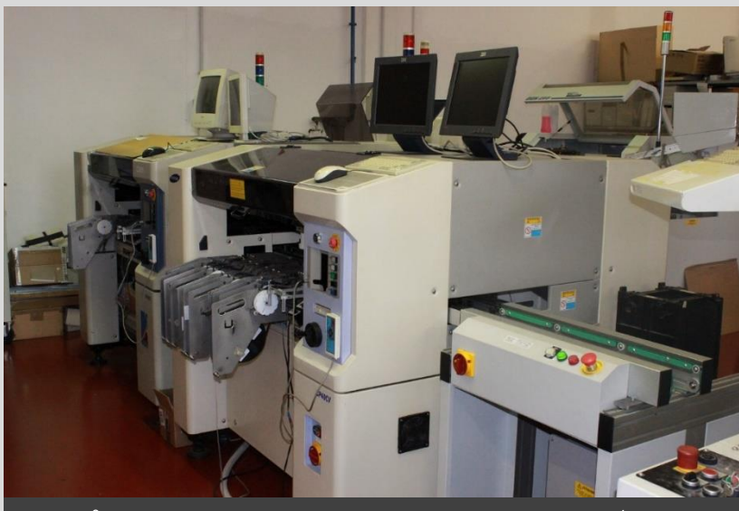
N° 2 PICK AND PLACE SAMSUNG CP40 5.000 COMP./ORA MONTAGGIO QFP/QFN/BGA/MICROBGA
