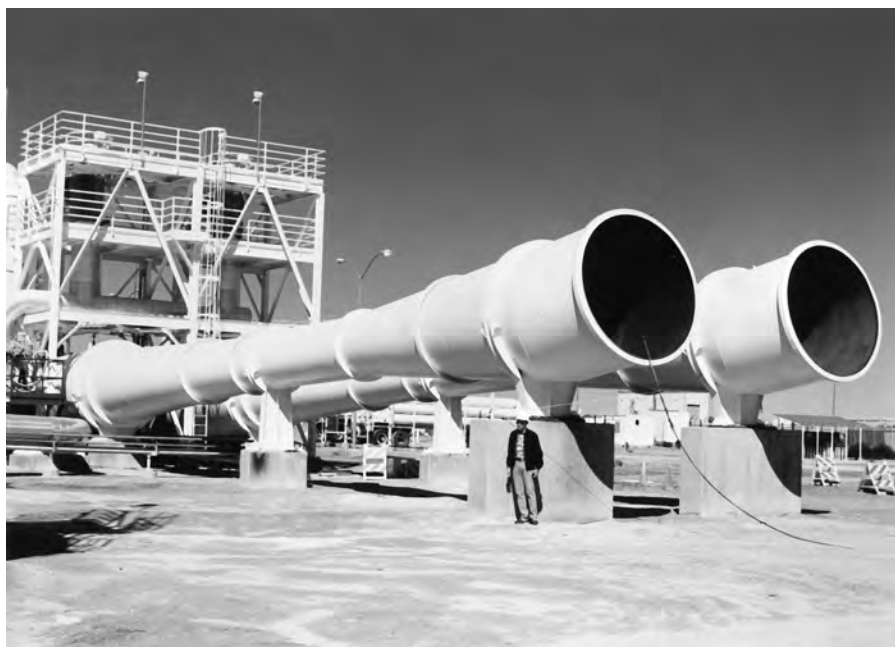
Fig. 33. These two steam jet ejectors serve as part of the pressure recovery system at the U.S. Army's high energy laser system test facility in White Sands, New Mexico. They are each 97 feet long with 96 inch diameter end-suction connections, and are among the largest ever manufactured anywhere. Each ejector handles a large quantity of low molecular weight gas at 120 Torr using the equivalent of 1.044 million pounds of steam per hour at 150 psig during the 14-second cycle.
