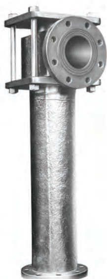
Fig. 12. Fig. 562 Steam Jet Ejector, constructed of impervious Graphite. Ejectors with 4" and above suction and pressure connections have fiberglass armoring. Nozzles are interchangeable with those used in the Fig. 555H Pump described on page 5.
