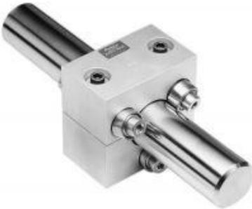
Zero- Max's Roh'Lix® linear actuators are threadless, mechanical, screw- type devices designed to convert rotary motion into precise linear motion and thrust using rolling element ball bearings. These adjustable automatic overload protectors will slip when overloaded, providing linear clutching without any additional clutch mechanisms.
