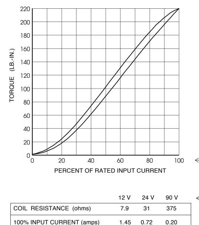
**CHARACTERISTICS** - With no electrical excitation, the shaft freely rotates. With electrical excitation, the shaft becomes coupled to the housing. Torque is proportional to input current (see torque graph), and independent of RPM. While the load torque is less than the output torque, the shaft won't rotate. When the load torque is increased, the brake will slip smoothly at the torque level set by the coil input current.
