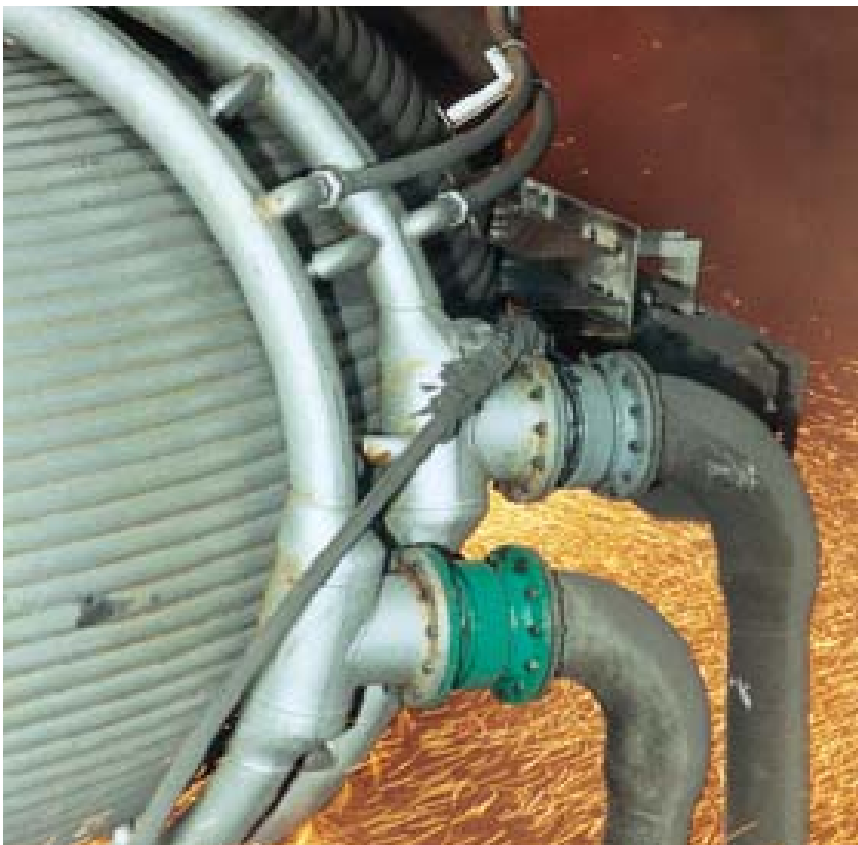
Type DG-02L basic unit with two-row ball bearing
